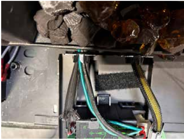
Diagram 7 Velcro affixed to IFC Tray
